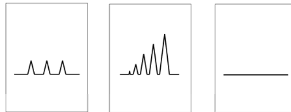
Fig. 5a-c: Different vibrotactile feedback conditions: Bumps , increasing and no-vibration .
