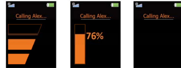
Fig. 3a-c: Different visualization techniques while placing a call: discrete , continuous , and blind .
