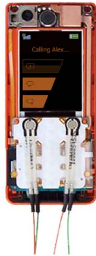
Fig. 1a,b: Callee phone (filter setup); Caller phone (call urgency selection, faceplate removed for illustrative purposes)
